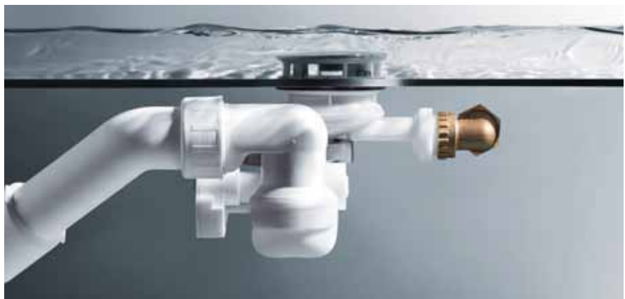
Compact construction height of only 110 mm. The designer bathtub fittings can be installed in bathtubs with a wall thickness between 3 and 10 mm and 52 mm and 90 mm drain holes. The rosette cover is made of chrome-plated brass
