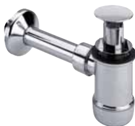
Odour Trap Entirely chrome-plated, for washbasins without overflow hole. Standpipe can be extended by 90 mm
