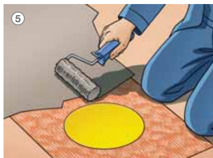
5 Work in the Schlüter-Kerdi sealing collar into the liquid foil.
